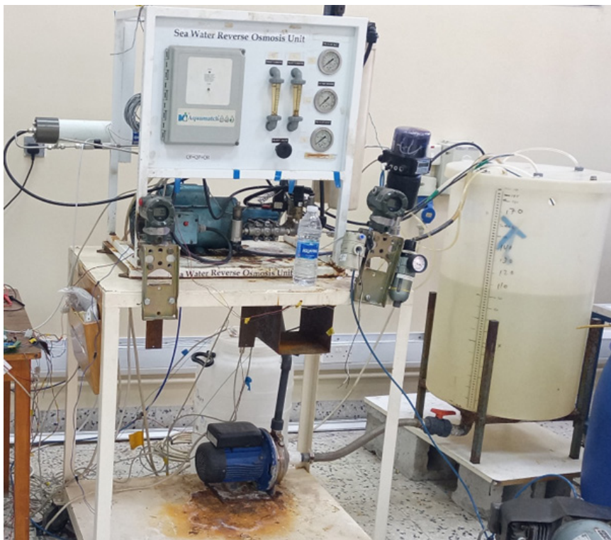
Fig.2 RO:1- membrane 2- visual pressure and flow 3- manual reject valve 4- reject control valve 5- diverting input flow control valve 6- feed flow transmitter 7- feed pressure transmitter 8- reject pressure transmitter 9- feed compressor 10- feed tank 11- reject flow transmitter 12- input pump 13- Mec10- sensor
